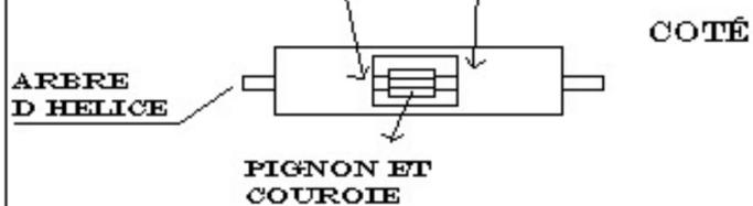
LA BAGUE EN NYLON M'EVITE LE FROTEMENT ENTRE LAITON ET LAITON
